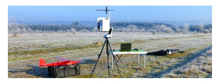
With a carry case, you can safely and easily move your ground station around the world. Running on rechargeable batteries, the ground station is designed to be very easy to use. The control interface has been developped following aeronautical codes and guarantees absolute safety. After a short training, the pilot will be comfortable with the interface, ready to operate the AVEM in all conditions.
